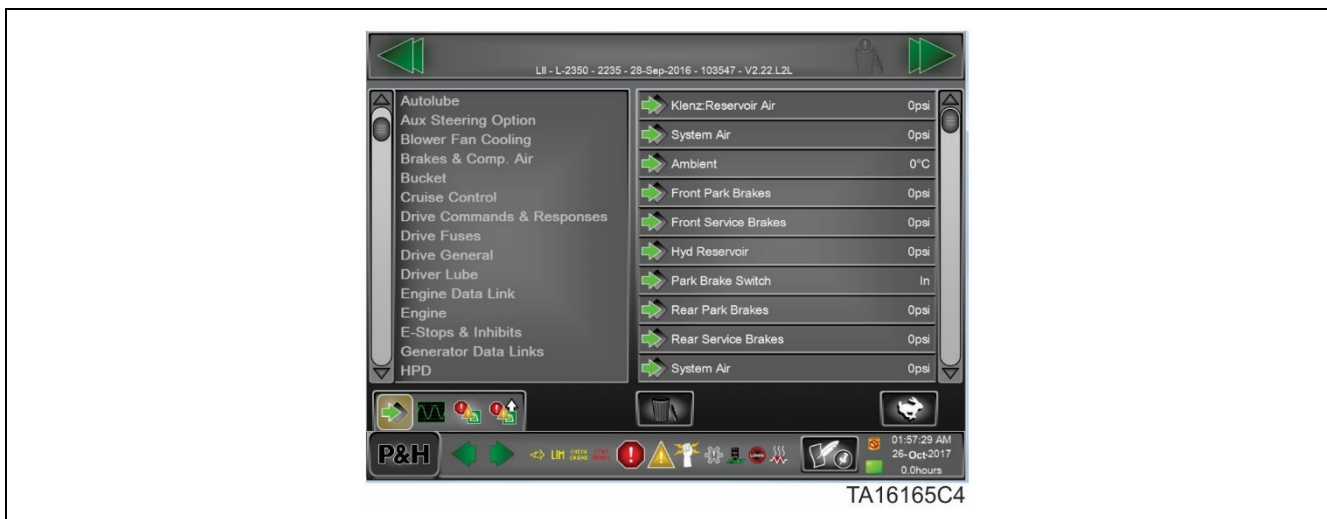
Figure 6. LINCS II channel selection screen (typical screen)
